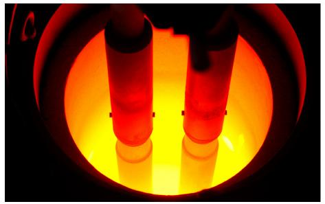
red reinforcing architectures and high starting levels of open porosity has been investigated as well. A dedicated process chain has been developed, based on various steps from the interphase coating of the ceramic fibres (TRL 3-4), and the fabrication of the porous CMC preforms by filament winding technique (TRL 3) up to the thermal treatment and the final non-destructive inspection of the samples.
